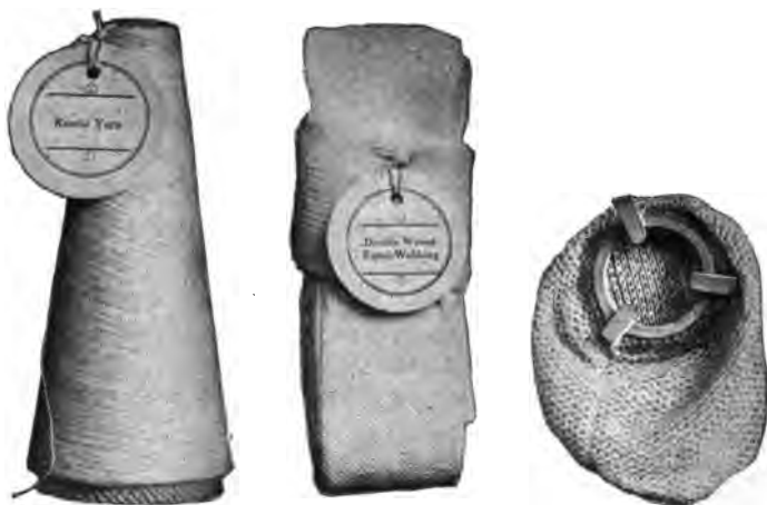
FIG. 29.—Welsbach gas mantles, showing how the fibers are woven and mounted.
